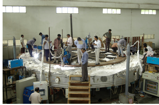
Fig IV: Hardfacing simultaneously by 4 PTAW machines
